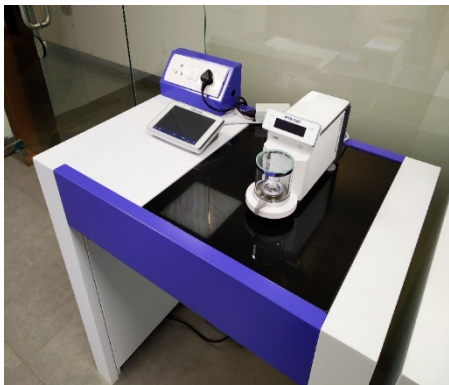
Mettler Toledo Micro Balance- XPR2 having readability of 0.001mg
