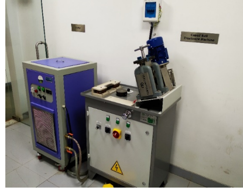
Cupell Ball Treatment Unit Italimpianti Orafi MSLR/B (339)
