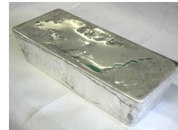
1000 oz Ag bar - uncontrolled shrinkage
