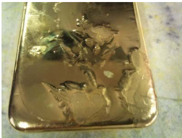
400 oz Au bar - dendrites, oxide formations and porosity
