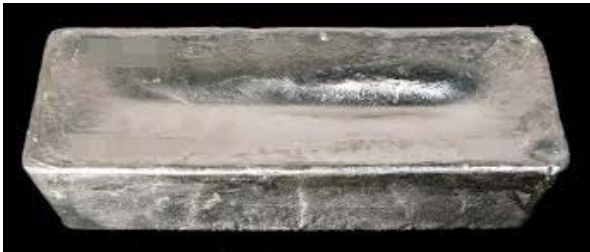
1000 oz Ag bar - central shrinkage hollow
