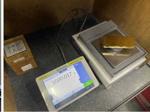
Every mass balance must have it's own dedicated calibration weight that itself is calibrated annually
