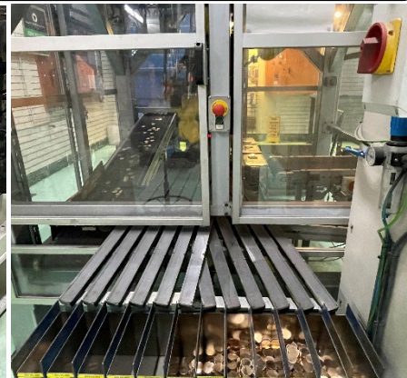
Coin weight sorting by robot
