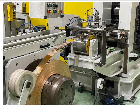
Precision strip rolling to 1micron for coins
