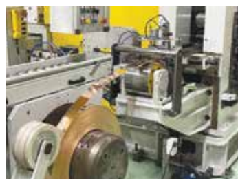
Precision strip rolling to 1micron for coins
