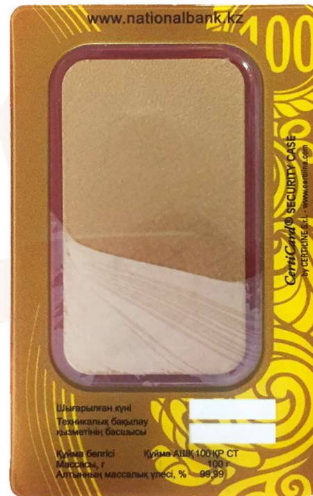
Inspection of the card back side in day light, after partial opening with loosing of the membrane trasparence and “FOG EFFECT”
